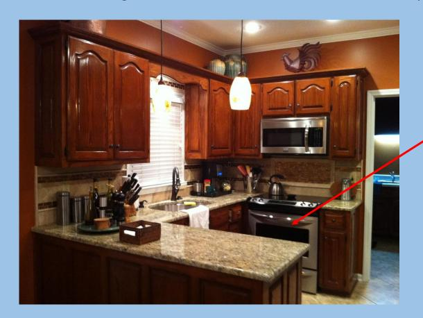
250V receptacle for the range would be required to be GFCI protected if within 6FT of the inside edge of the sink.
